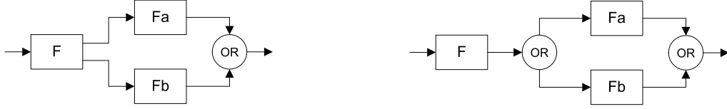
Figure 2.1: Non-decomposed, multi-exit function and its single-exit equivalent
